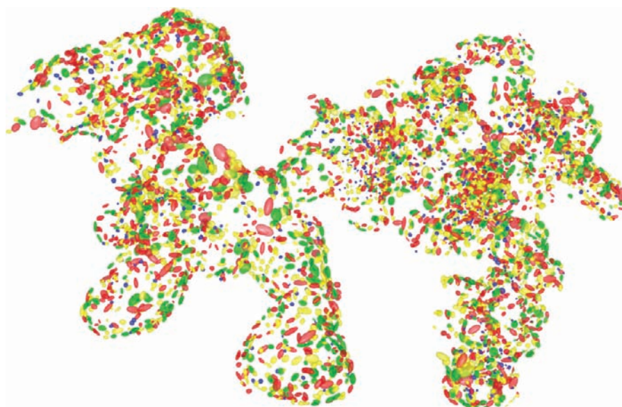
Figure 7. Spatial distribution of the fitted ellipsoids. Green: oblate, red: prolate, yellow: indistinguishable, blue: spherical within the error limits. The particle density is higher on the right side.
